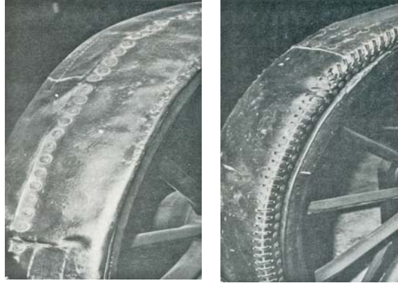
Replicas of Thomson's original leather-covered carriage tire owned by the British Science Museum are among the last known examples of the earliest pneumatics. Tire at left is held together by rivets, which Thomson believed would also aid traction. Leather covering at right is laced together.
